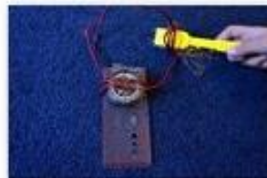
Notice the compass arrow in the top picture and that it has moved in the picture to the right! As the magnet moves near the wire, the electrons in the wire move from atom to atom.
